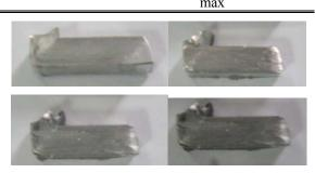
**Fig. 1.** ECAP samples after 1(a), 2(b), 3(c), and 4(d) passes
