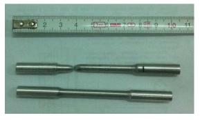
Fig. 2. Shape of the specimen before and after the tensile test, for commercially pure A6063
